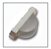
For an LED to light properly, the amount of current that flows through it needs to be controlled. To do this we usually use a current limit resistor. If we didn't, the LED would probably be very bright for a short amount of time, before being permanently destroyed.
