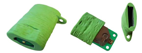
In the second example, the case uses laser cut rubber to create a complete shell around the torch, with a slot at one end to allow the LED light to shine out. The case is made up of segments which are glued together and then slotted over the torch PCB.
