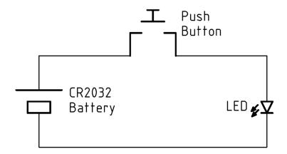
The circuit diagram for the torch is shown above. It is a very simple circuit, powered by a CR2032 coin cell battery.
