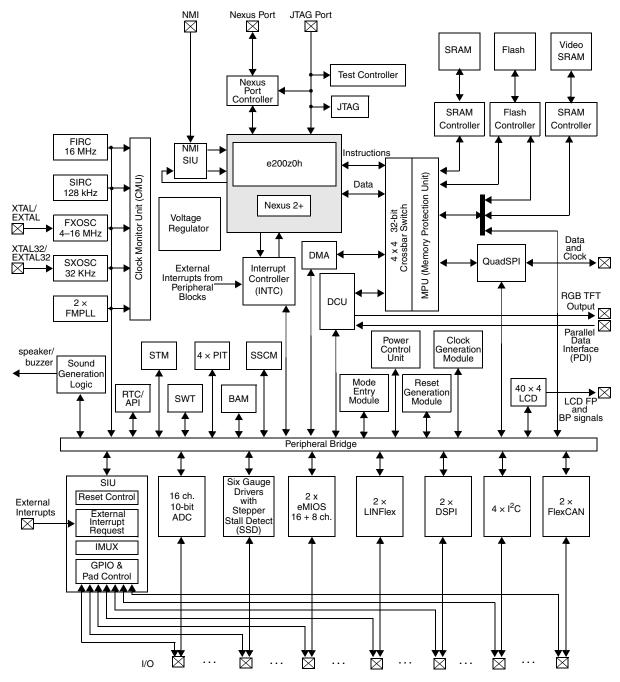
Figure 1. MPC5606S block diagram
