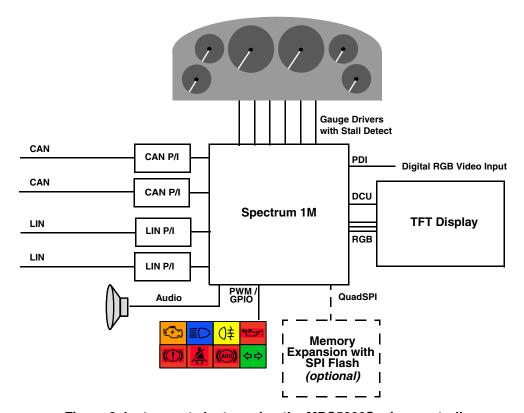
Figure 2. Instrument cluster using the MPC5606S microcontroller
