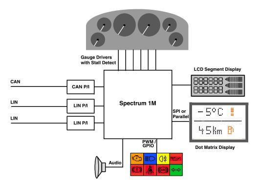
Figure 3. Instrument cluster using MPC5606S
