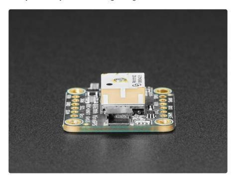
Best of all, we added all the extra goodies you could ever want: a ultra-low dropout 3.3V regulator so you can power it with 3.3-5VDC in, 5V level safe inputs on UART and I2C, a footprint for optional CR1220 coin cell to keep the RTC running and allow warm starts, a green power LED and a tiny red PPS LED. The LED blinks at about 1Hz when a fix is found and is off when no fix.
