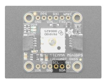
SCL - this is the I2C clock pin, connect to your microcontroller or computer's I2C clock line.
