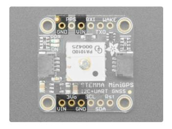
VIN - power input, connect to 3-5VDC. It's important to connect to a clean and quiet power supply. GPS's are very sensitive, so you want a nice and quiet power supply. Don't connect to a switching supply if you can avoid it, an LDO will be less noisy! This module only draws 30mA current during navigation
