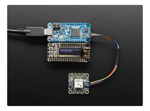
This miniature GPS breakout is only 1"  $\times$  1" ( $^{\sim}$  25mm  $\times$  25mm) but houses a complete GPS/GNSS solution with both I2C and UART interfaces. There's even an antenna on top so it's plug and play!
