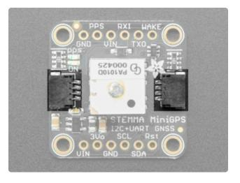
On both sides in the middle are the Sparkfun Qwiic () compatible STEMMA QT () JST SH connectors, for using with I2C. Use with any of the STEMMA QT cables available in the Adafruit shop to connect this breakout to your project without needing to solder!
