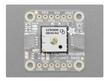
The PA1010D GPS module with built-in antenna is located in the center of the board. It has all kinds of features!
