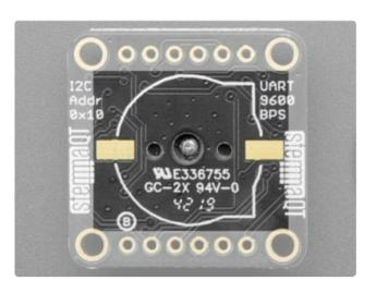
The back has a footprint for an optional coin cell battery. The board ships with a CR1220 coin cell holder that can be soldered onto the back. CR1220 battery not included.
