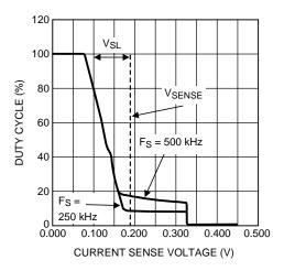
Figure 30. Current Sense Voltage vs Duty Cycle
