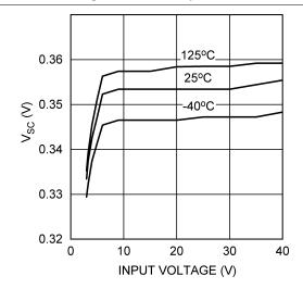
Figure 16. Short Circuit Sense Voltage vs Input Voltage
