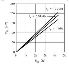
Figure 17. Compensation Ramp vs Compensation Resistor
