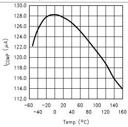
Figure 15. COMP Pin Source Current vs Temperature
