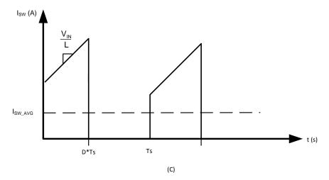
Figure 29. Inductor Current and Diode Current
