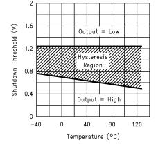
Figure 18. Shutdown Threshold Hysteresis vs Temperature
