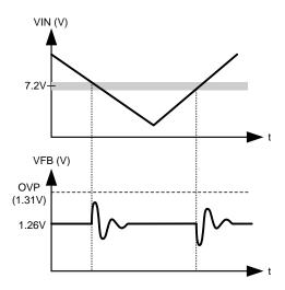
Figure 21. The Feedback Voltage Experiences an Oscillation if the Input Voltage crosses the 7.2-V
