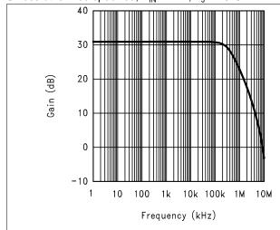
Figure 13. Error Amplifier Gain
