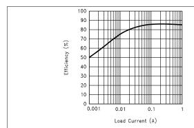
Figure 35. Efficiency vs Load Current (3.3-V In and 12-V Out)
