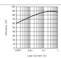
Figure 36. Efficiency vs Load Current (5-V In and 12-V Out)
