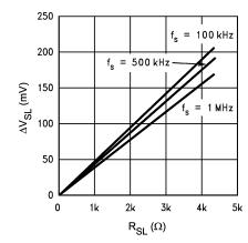
Figure 24. External Slope Compensation  $\Delta V_{SL}$  vs  $R_{SI}$
