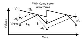
Figure 22. Sub-Harmonic Oscillation for D>0.5 and Compensation Ramp to Avoid Sub-Harmonic Oscillation
