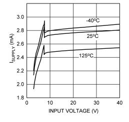
Figure 1.  $I_Q$  vs Input Voltage (Shutdown)
