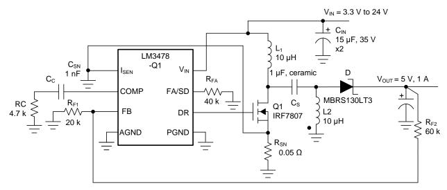
Figure 34. Typical SEPIC Converter
