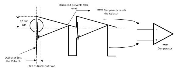
Figure 20. Basic Operation of the PWM Comparator
