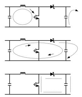
Figure 37. Current Flow in a Boost Application
