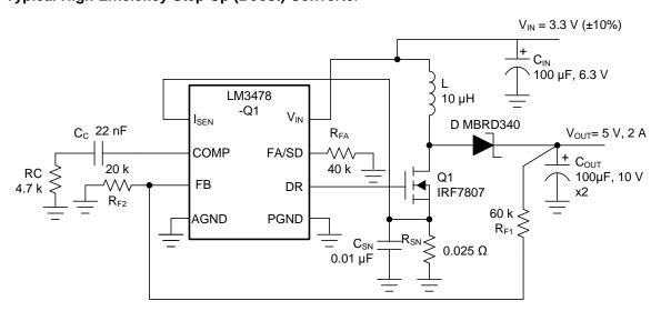
Figure 27. Typical High Efficiency Step-Up (Boost) Converter Schematic
