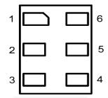
Figure 2. Pad Assignments (Top-Through View)
