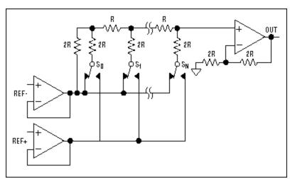
Figure 1. Simplified DAC circuit.
