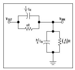
Figure 6. Equivalent circuit of feedback network.
