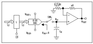
Figure 3. An improved deglitch circuit.
