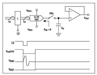
Figure 2. Integrated T/H deglitch architecture.
