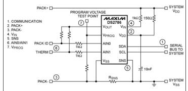
Figure 1. Circuit board nodes that must be verified.
