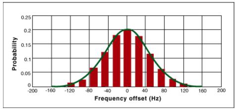
Figure 3. The probability distribution of frequency estimate error.
