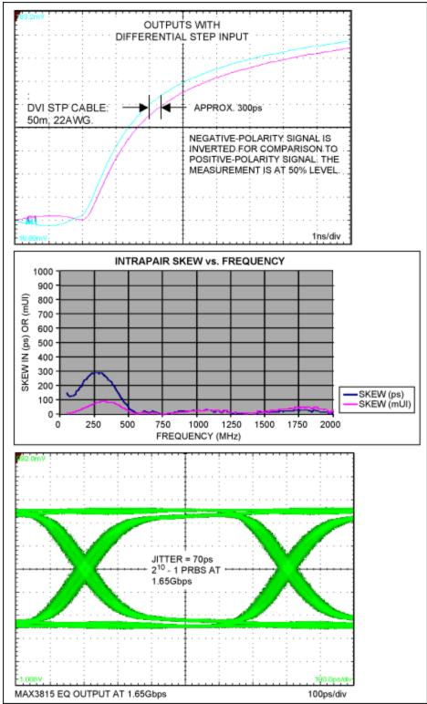
Figure 3. Step method fails to predict serial data jitter.
