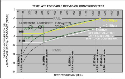
Figure 10. Simplified test template, with underlying family of curves shown for fundamental-only and multipleharmonic cases.
