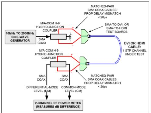
Figure 12. This test setup features a low-cost generator, couplers, and power meters.
