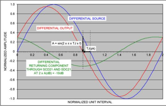
Figure 6. Offset in the zero-crossing time TJ(pk) is caused by SCD21 and SDC21. All waveforms shown are differential signaling (single ended not shown).
