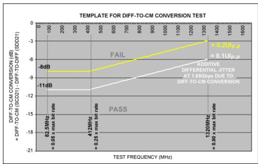
Figure 9. Simplified test template, for which 0.1UIP-P pass/fail criteria are recommended.
