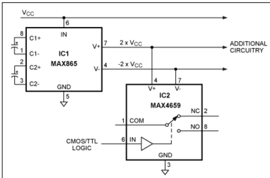
Figure 1. The MAX865 dual-output charge pump (IC1) provides a local bipolar power supply for the MAX4659 CMOS analog switch (IC2).
