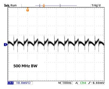
Output Ripple:  $V_{IN}$  = 3.3V,  $V_{OUT}$  = 1.0V, lout = 400mA
