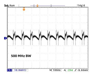
Output Ripple: V<sub>IN</sub> = 5V, V<sub>OUT</sub> = 1.0V, Iout = 400mA C<sub>IN</sub> = 2.2μF/0603, C<sub>OUT</sub> = 10μF/0603 + 2.2uF/0603
