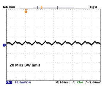
Output Ripple: V<sub>IN</sub> = 3.3V, V<sub>OUT</sub> = 1.0V, Iout = 400mA
