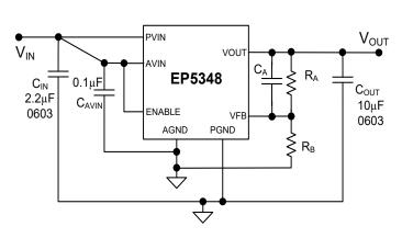
**Figure 1: Simplified Applications Circuit**
