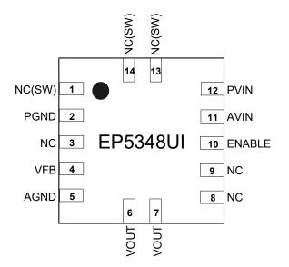
Figure 3: EP5348UI Pin Out Diagram (Top View)
