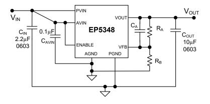
Figure 4. EP5348UI Application Circuit
