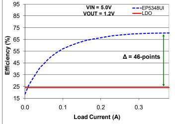
Figure 2: Highest Efficiency in Smallest Solution Size
