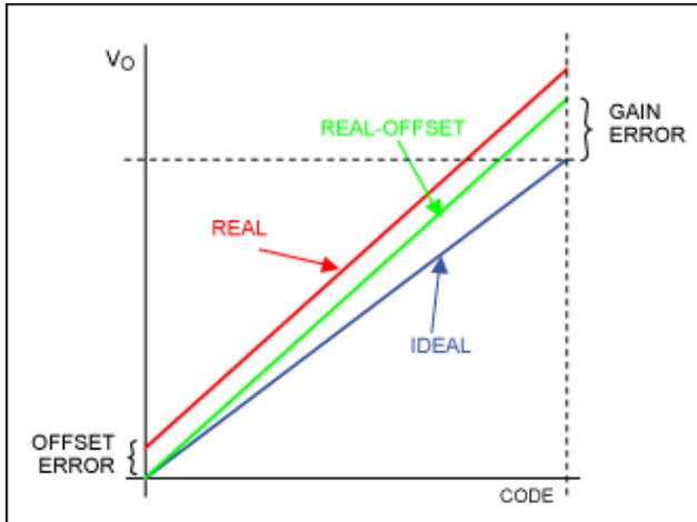
Figure 1. Gain and offset errors.
