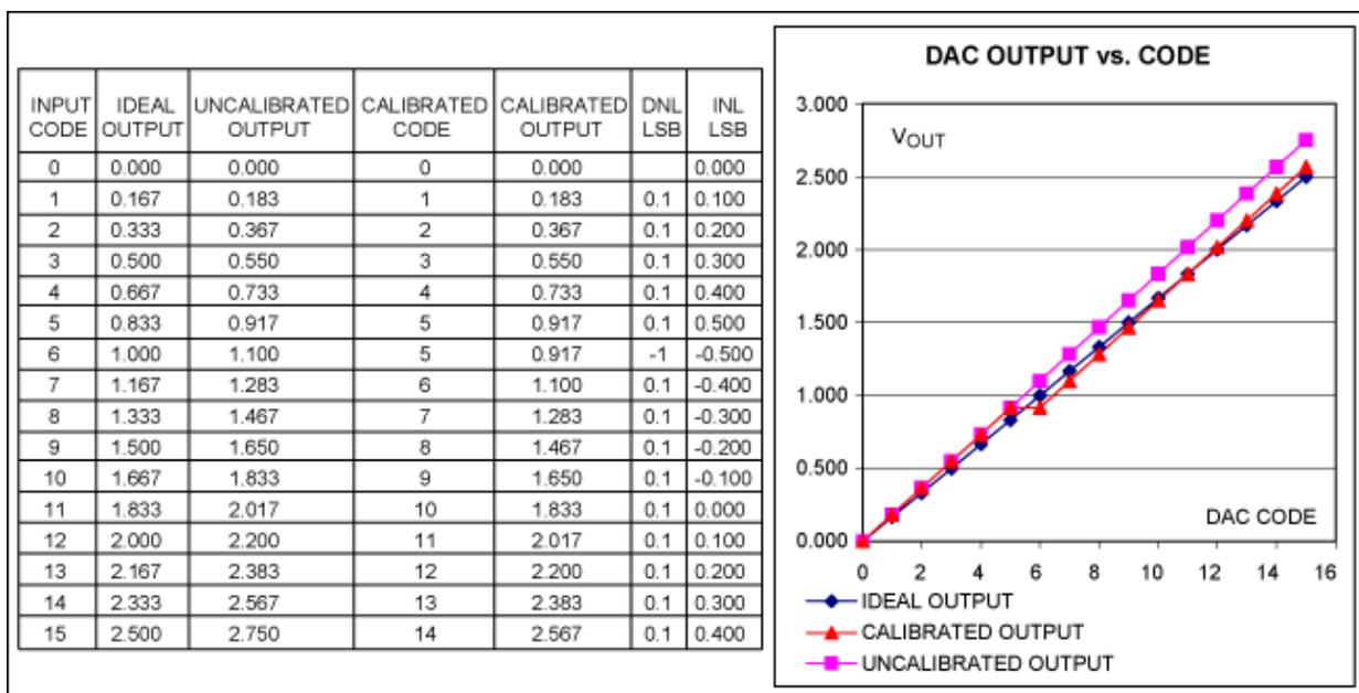
Figure 3. A digitally calibrated DAC system.
