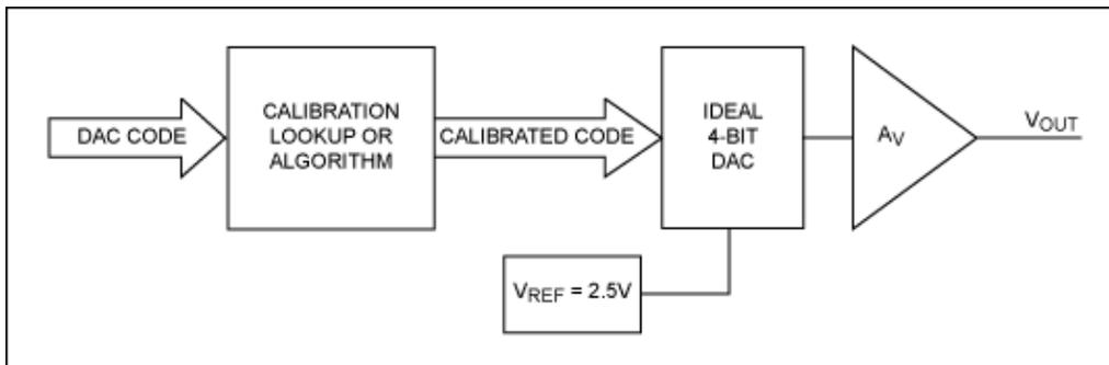
Figure 2. System to demonstrate digital gain calibration.
