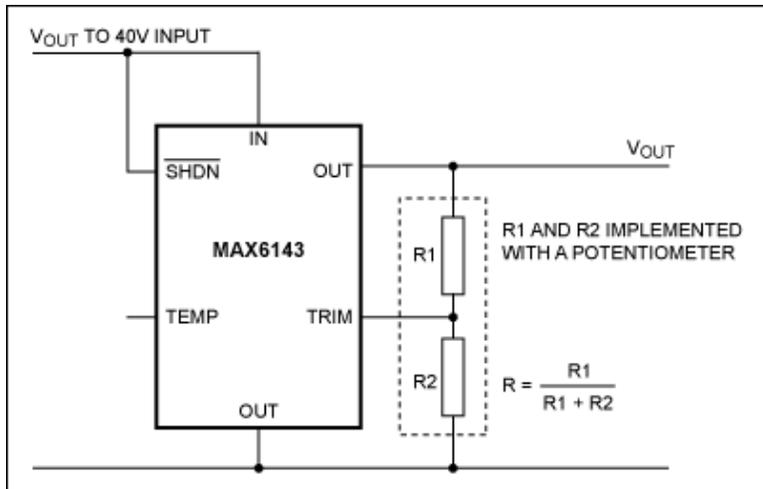
Figure 4. Typical operating schematic for the MAX6143.
