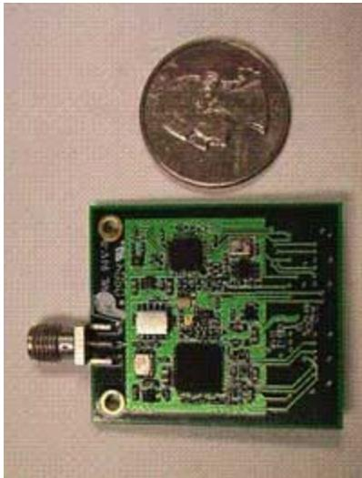
Figure 2. TD-SCDMA reference design board.
