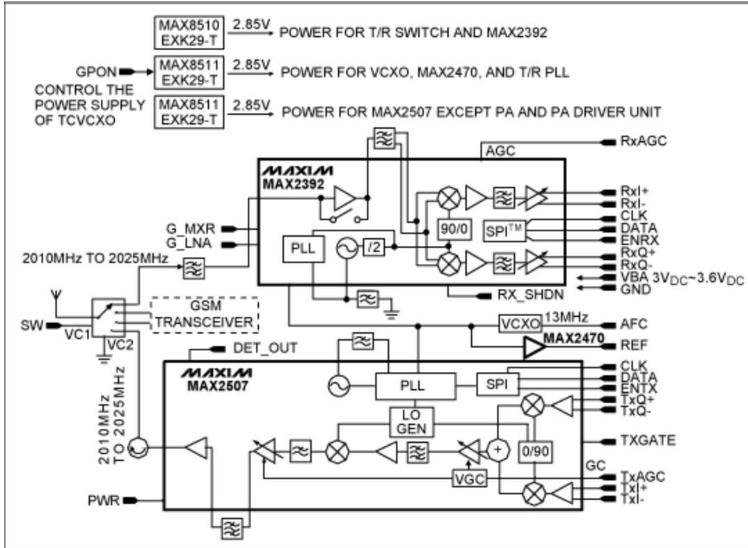
Figure 1. TD-SCDMA reference-design functional block diagram.
