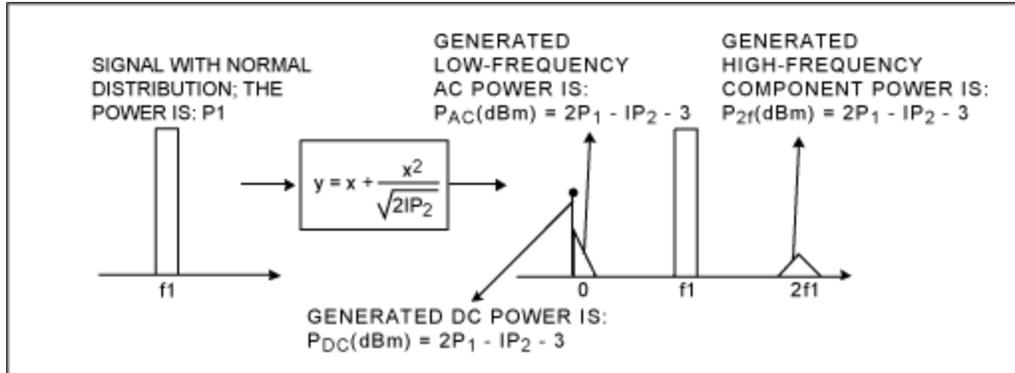
Figure 4. 2nd-order intermodulation products.
