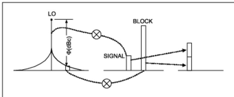
Figure 5. Reciprocal mixing of LO phase noise onto an interferer.
