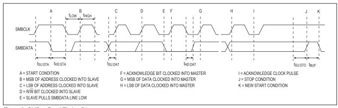
Figure 3. SMBus Read Timing Diagram
