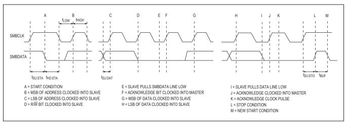
Figure 2. SMBus Write Timing Diagram
