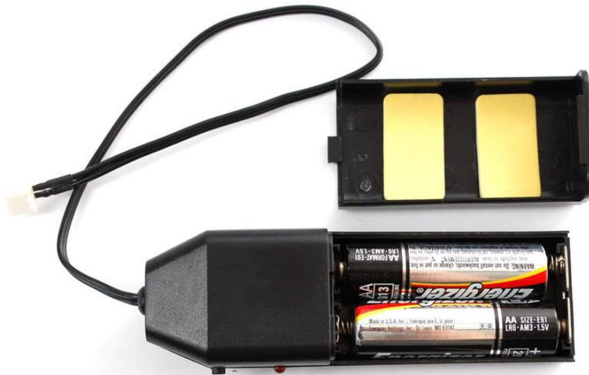
This pocket inverter can drive approximately 1 to 15 feet (0.3-5 meter) of 'classic' EL wire such as LyTec. Since we are using higher-brightness EL wire in the shop, it can only drive half as much, 1 to 7.5 feet (0.3 to 2.5 meter). We found that 2 meters gives a nice bright glow at good voltage and frequency. At 3 meters, its not as bright, it appears about the same as 'classic' EL.
