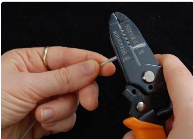
Next, we'll need to remove the outer coating. This is the hardest part of the process so don't be disappointed if it takes a few tries to get it right! Use the 20 AWG or 18 AWG slot and strip off the PVC coating about 1/2" (1 cm) away from the end.
