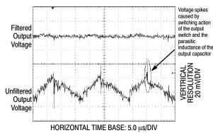
Figure 21. Output Ripple Voltage Waveforms
