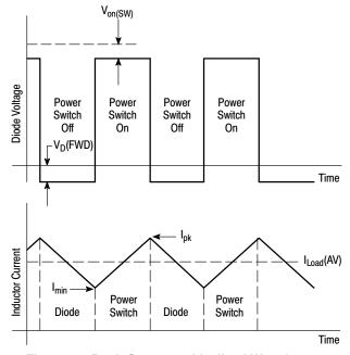
Figure 17. Buck Converter Idealized Waveforms
