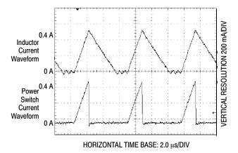
Figure 20. Discontinuous Mode Switching Current Waveforms
