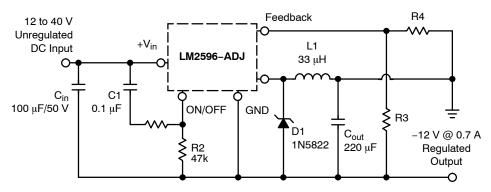
Figure 23. Inverting Buck-Boost Develops -12 V
