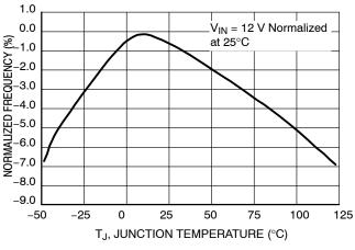
Figure 10. Switching Frequency
