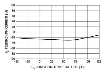
Figure 12. Feedback Pin Current
