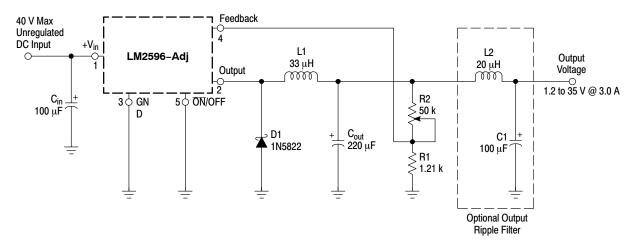
Figure 30. 1.2 to 35 V Adjustable 3.0 A Power Supply with Low Output Ripple
