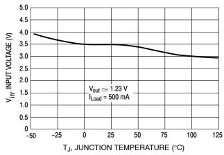
Figure 11. Minimum Supply Operating Voltage
