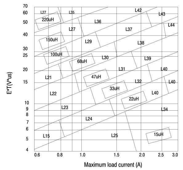
Figure 18. Inductor Value Selection Guides (For Continuous Mode Operation)
