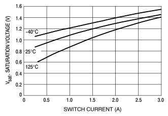
Figure 9. Switch Saturation Voltage
