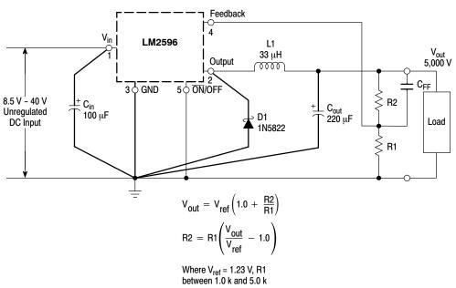
Figure 15. Typical Test Circuit
