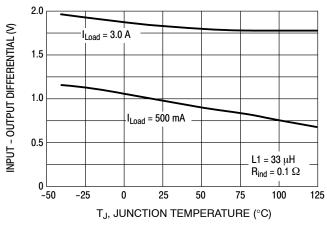
Figure 4. Dropout Voltage
