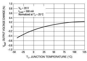
Figure 2. Normalized Output Voltage
