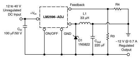
Figure 22. Inverting Buck-Boost Develops -12 V
