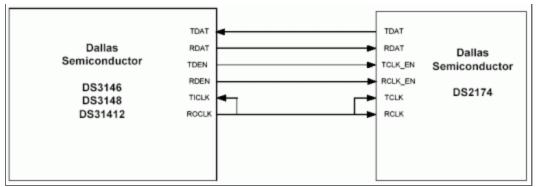
Figure 1. Ungapped clock mode BERT and framer bidirectional synchronization.
