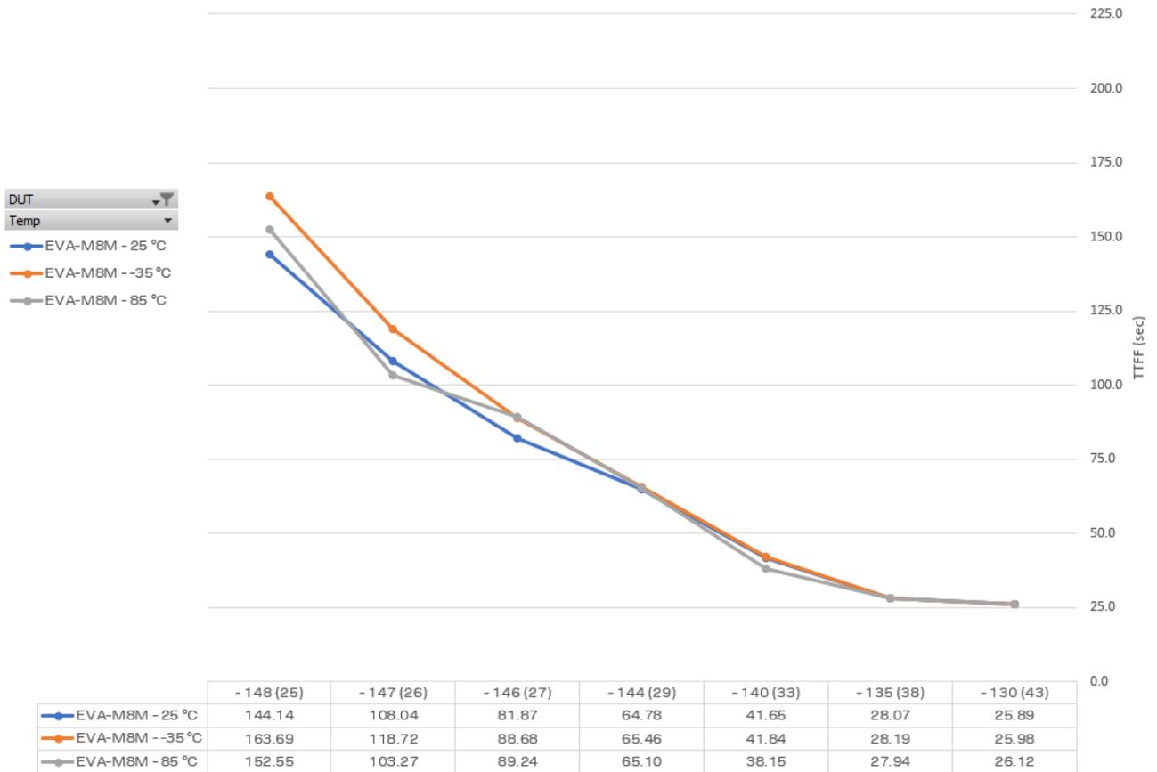
**Figure 3: TTFF vs. signal power for EVA-M8M during cold starts at +25, -35, and +85 °C (default mode: GPS & GLONASS including QZSS, SBAS)**
