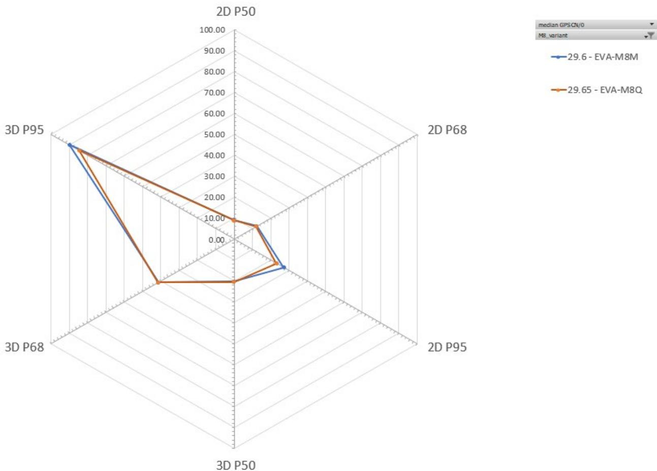
**Figure 6: Position error in meters for EVA-M8Q and EVA-M8M in percentiles. Urban canyon with good and bad signal reception conditions (default mode: GPS and GLONASS including QZSS, SBAS)**
