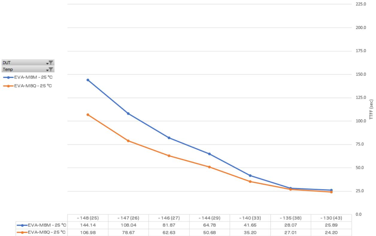
**Figure 2: TTFF vs. signal power for EVA-M8Q and EVA-M8M during cold starts<sup>10</sup> (default mode: GPS & GLONASS including QZSS, SBAS)**
