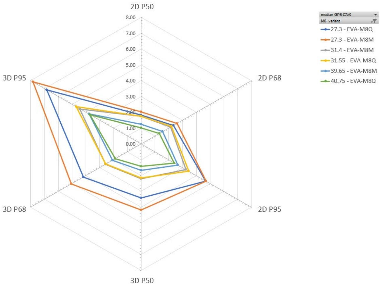
**Figure 5: Position error in meters for EVA-M8Q and EVA-M8M in percentiles at 27.3, 31.5 and 40 dBHz in rural areas (default mode: GPS and GLONASS including QZSS, SBAS)**
