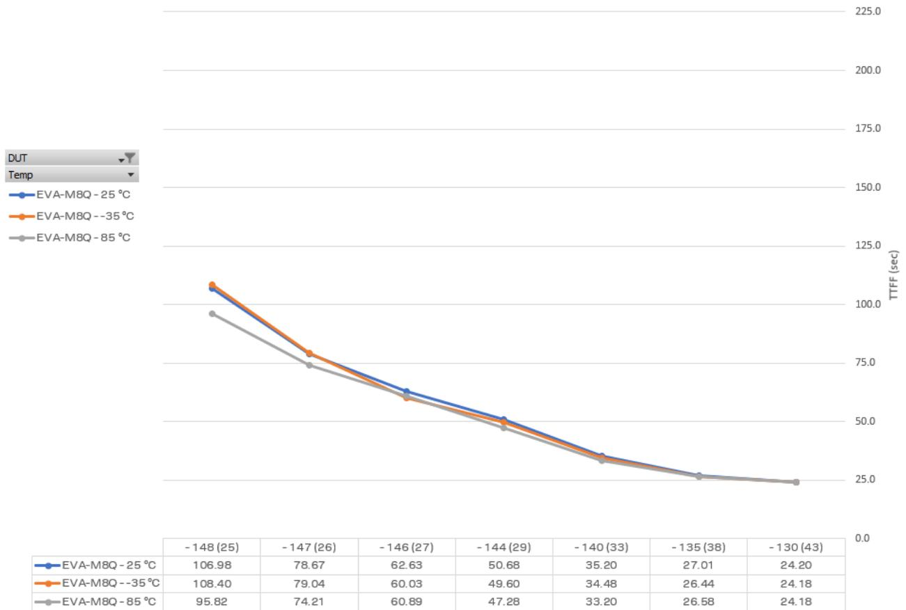
**Figure 4: TTFF vs. signal power for EVA-M8Q during cold starts at +25, -35, and +85 °C (default mode: GPS & GLONASS including QZSS, SBAS)**
