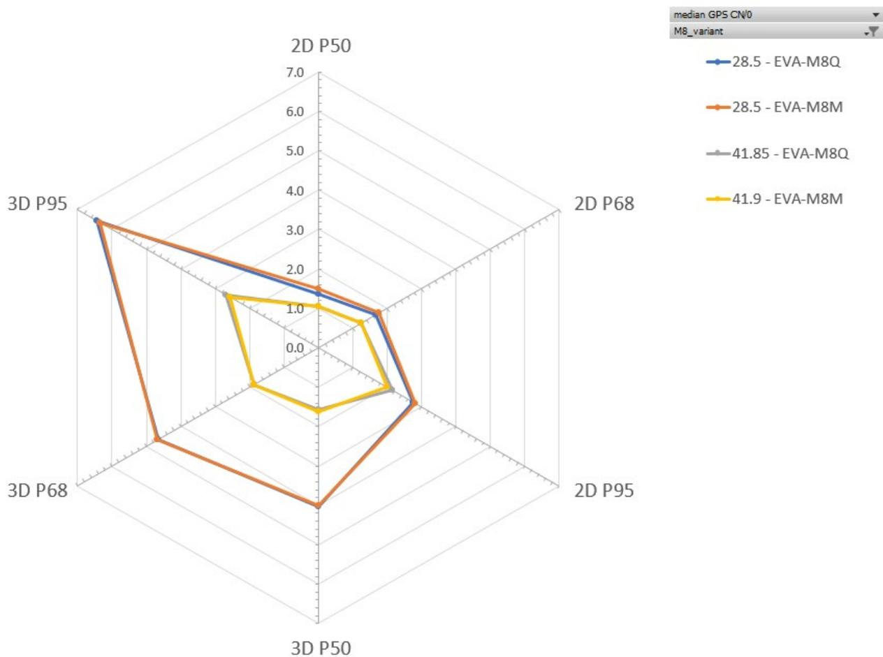
Figure 9: Position error in meters for EVA-M8Q and EVA-M8M in percentiles. Highway with strong and weak signal reception conditions (default mode: GPS and GLONASS including QZSS, SBAS)
