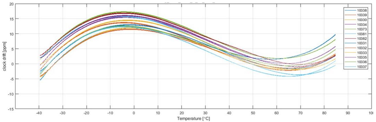
Figure 1: Temperature effect on crystal on various crystal-based modules
